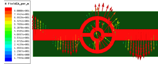
Fig. 6 – Cross shaped BPFs H -field distribution
