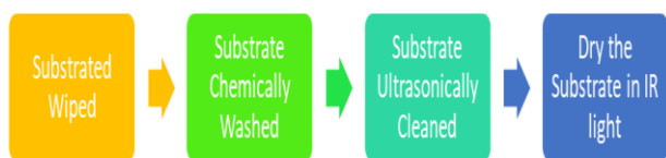
Fig. 1 – The procedure employed for substrate cleaning
