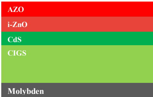
Fig. 1 – The Ultrathin CIGS solar cell structure
