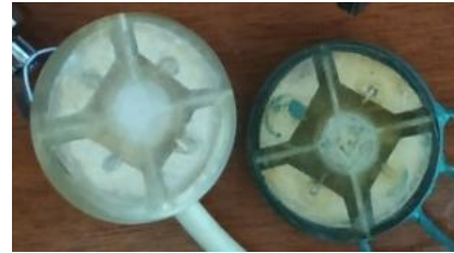
Fig. 9 – Appearance of the outer and inner parts of the created model of a cochlear implant with an acoustic information transmission channel
