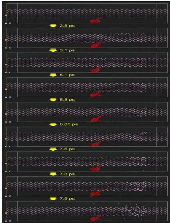
Fig. 5 – The evolution of the destruction of the p-n junction under simultaneous influence of the thermal and electromagnetic components of the pulse
