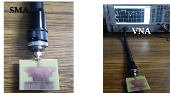
Fig. 4 – Measurement and testing blocks of the manufactured MS-integrated patch antenna
