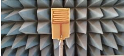
Fig. 7 – The measurement configuration for the patch antenna
