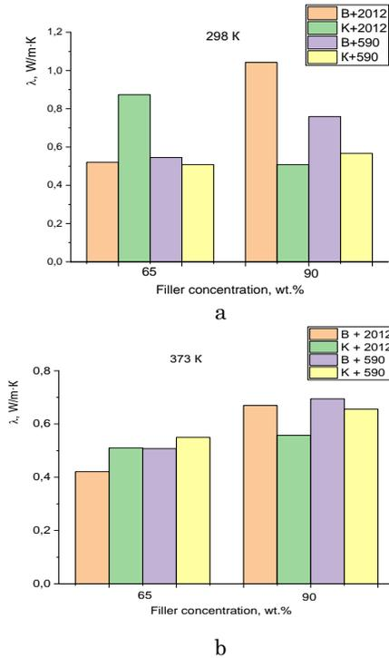
Fig. 2 – Dependence of thermal conductivity on filler concentration (at different temperatures) for the studied systems
