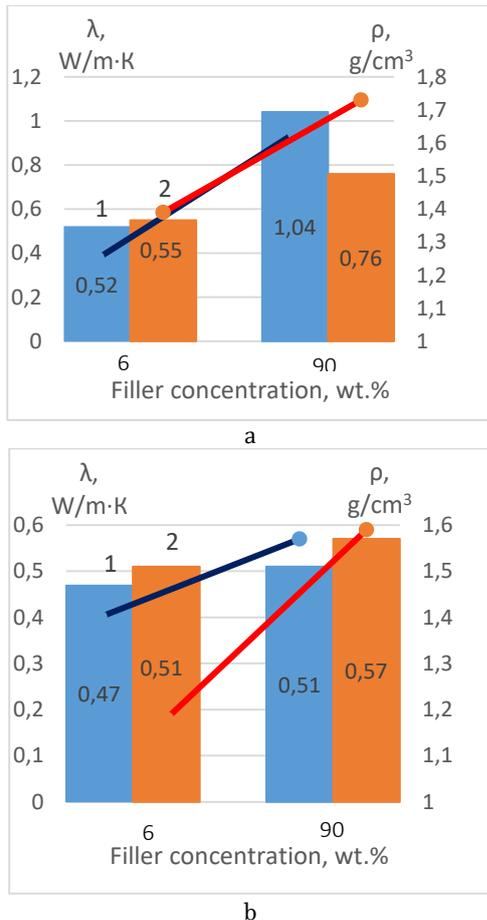
Fig. 3 – Dependence of thermal conductivity coefficient and composite density for systems with Ash B (a) and Ash K (b): 1 – Latex 2012, 2 – Policril 590
