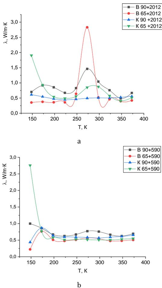
**Fig. 1** – Dependence of the thermal conductivity coefficient on temperature for the studied systems based on Latex 2012 (a) and Policril 590 (b)
