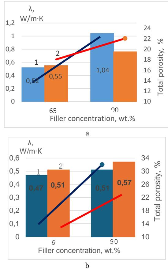
Fig. 4 – Dependence of thermal conductivity and total porosity for composites with Ash B (a) and Ash K (b) in systems based on: 1 – Latex 2012, 2 – Policril 590
