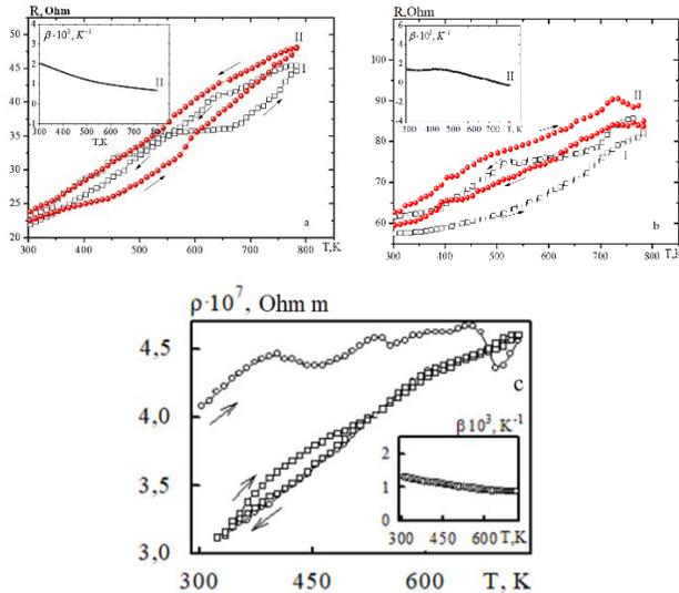
**Fig. 2** – Temperature dependence of resistance (a, b) and resistivity (c) and TCR for film systems: a – phase  $\text{Fe}_3\text{Pt}$ , film thickness 80 nm; b – phase  $\text{FePt}$ , film thickness 50 nm; c – phase  $\text{Ni}_3\text{Mo}$ , film thickness 70 nm
