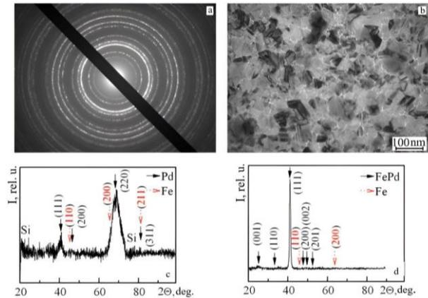
**Fig. 1** – Diffraction pattern (a), microstructure (b) and X-ray diffraction patterns from the film alloy FePd/S
