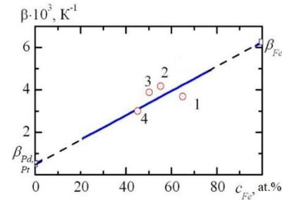
**Fig. 3** – Concentration dependence of TCR for film systems: 1 – phase  $\text{FePd}$  ( $d = 10$  nm); 2 –  $\text{FePd}$  ( $d = 15$  nm); 3 – phase  $\text{FePt}$  ( $d = 15$  nm); 4 – phase  $\text{FePd}$  ( $d = 20$  nm). Magnitudes  $\beta_{\text{Pd}}$ ,  $\beta_{\text{Pt}}$  and  $\beta_{\text{Fe}}$  correspond to thickness films 20 nm
