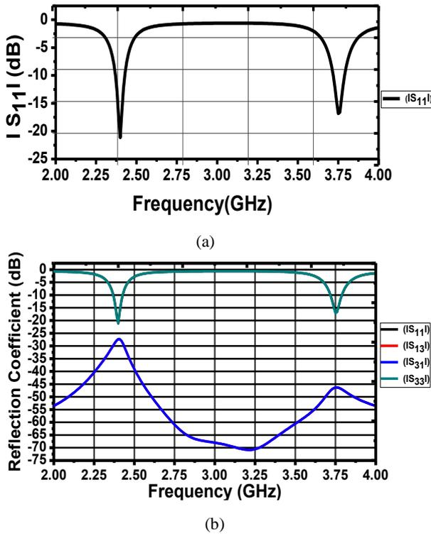
Fig. 5 – S-Parameters: (a) Reflection coefficient, (b) Isolation
