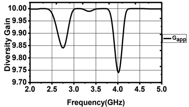
Fig. 12 – The measured diversity gain of proposed MIMO
