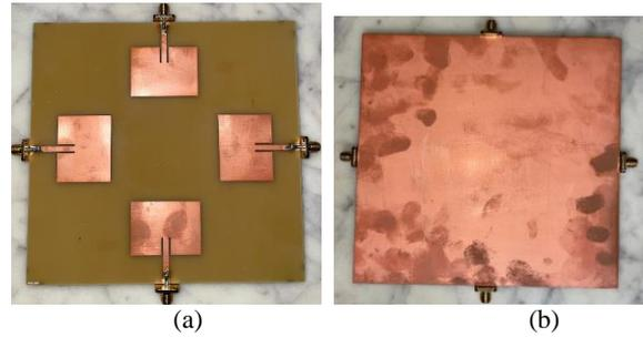
Fig. 11 – Fabricated model of proposed antenna: (a) Front view, (b) Back view
