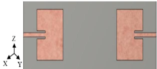
Fig. 4- Two radiators Geometry with distance 60.6mm
