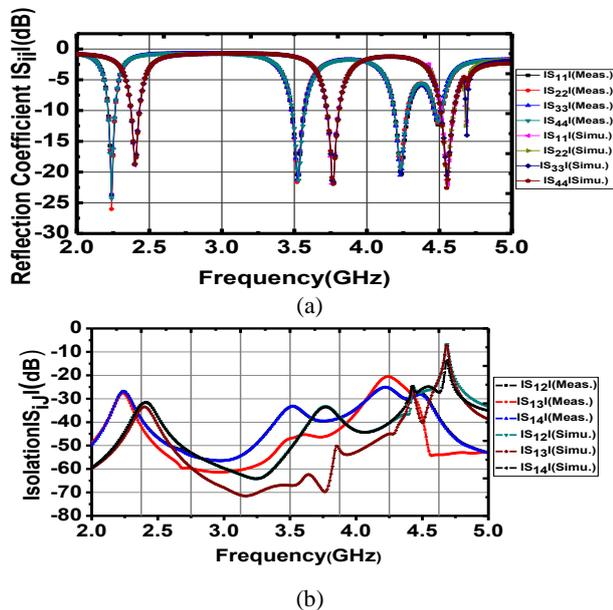
Fig. 10 – S-parameters of presented MIMO (a) Reflection coefficient (b) Isolation
