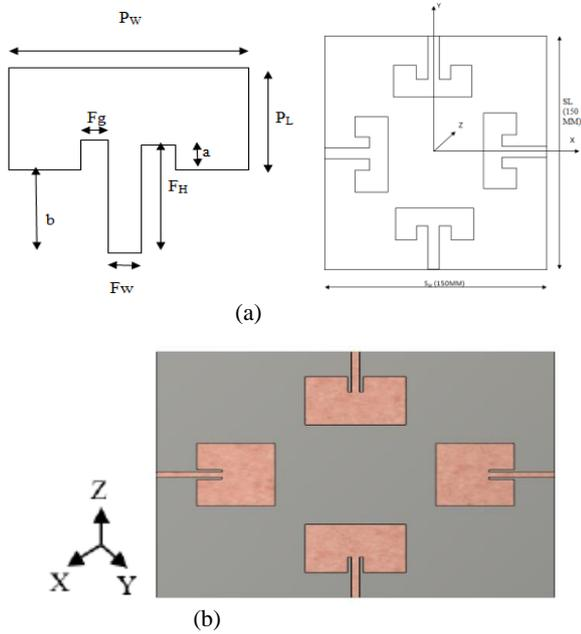
Fig. 1 – Proposed antenna Geometry: (a) patch view with dimensions (b) four port view
