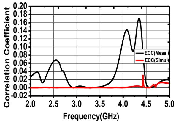
Fig. 13 – Comparison of measured and simulated ECC
