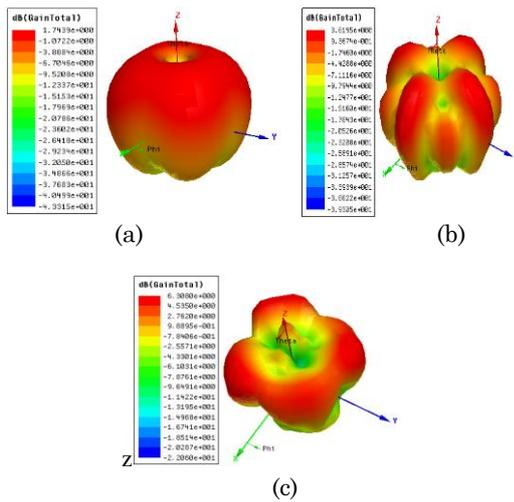
Fig. 15 – 3D radiation pattern at: (a) 2.4 GHz, (b) 3.7 GHz (c) 3.5 GHz
