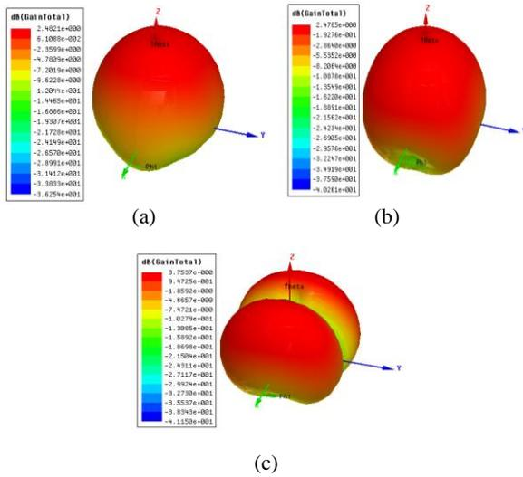
Fig. 6 – Radiation pattern 3D at 2.4 GHz: (a) Port-1, (b) Port-2 (c) Port 1 and 2
