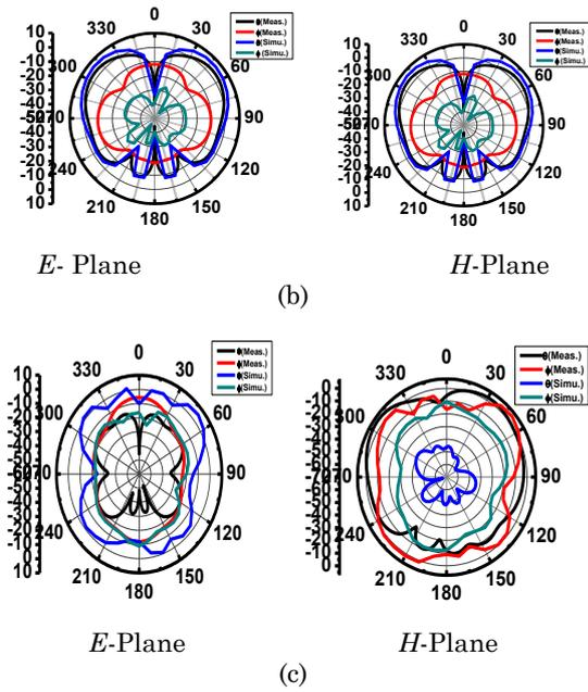
Fig. 14 – Radiation pattern at (a) 2.4 GHz, (b) 3.7 GHz (c) 4.5 GHz
