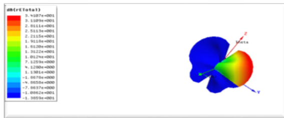
Fig. 6 – Designed antenna array's 3D far-field emission patterns
