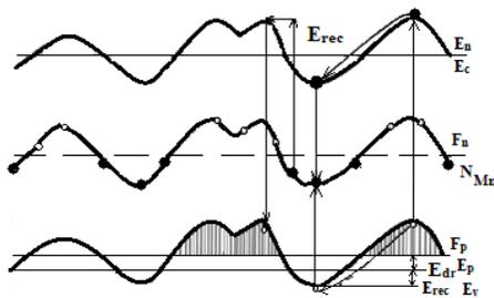
**Fig. 3** – Zone diagram of compensated silicon doped with impurity manganese atoms based on the model of inhomogeneous semiconductor
