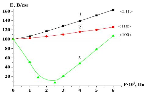
**Fig. 1** – Variation of threshold electric field strength in silicon doped with impurity manganese atoms with different crystallographic directions as a function of uniaxial pressure, at  $T = 80 \text{ K}$ ,  $I_f = 30 \text{ lux}$
