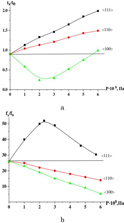
**Fig. 2** – Dependences of the amplitude (a) and frequency (b) of current auto-oscillations on the value of uniaxial elastic compression  $P$  for silicon samples doped with impurity manganese atoms with different crystallographic directions  $\langle 111 \rangle$ ,  $\langle 110 \rangle$  and  $\langle 100 \rangle$  at  $E = 250 \text{ V/cm}$ ,  $I_0 = 9 \text{ mA}$ ,  $f_0 = 0.2 \text{ Hz}$
