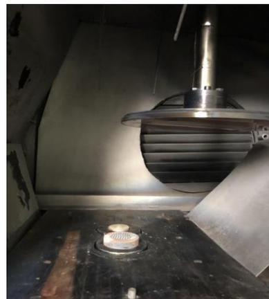
**Fig. 1** – The technological scheme of obtaining of CM NaCl-Fe by the EB-PVD method (a) and technological chamber of the laboratory EB-installation UE-150: 1 – substrate; 2 – condensate (CM); 3 – EB-guns; 4 – vapor flow; 5 – Fe-ingot; 6 – NaCl-tablet; 7 – reactor for NaCl evaporating; 8 – input tube of vacuum system (to vacuum pump)
