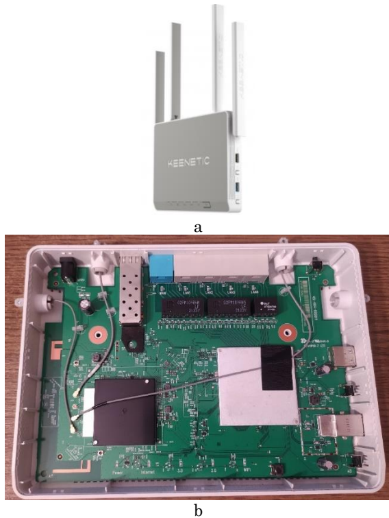
Fig. 2 – Router KN-1011: general appearance (a), printed circuit board (b)
