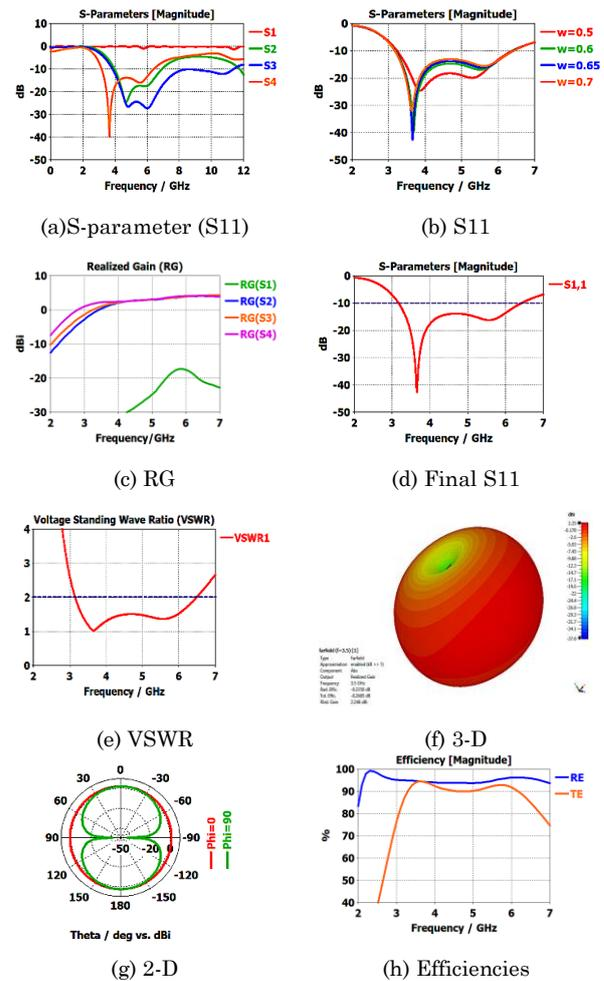
**Fig. 3** – The antenna design performance parameters of the SEA
