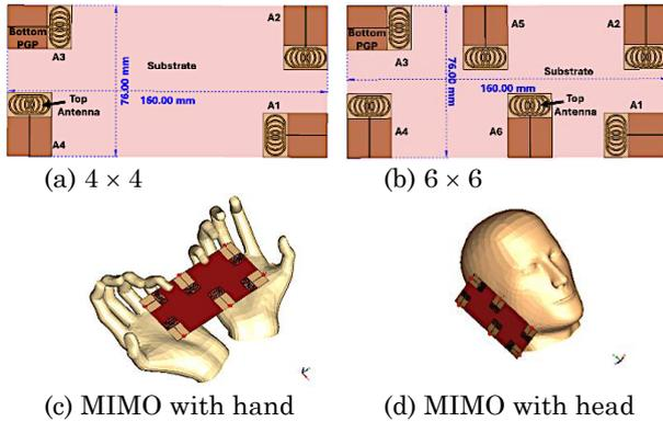
**Fig. 2** – The MIMO layouts and the setups for the SAR calculation
