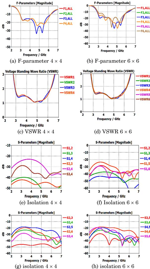
Fig. 4 – The F-parameter, VSWR and the Isolation characteristic of the  $4 \times 4$  and  $6 \times 6$  MIMO arrays
