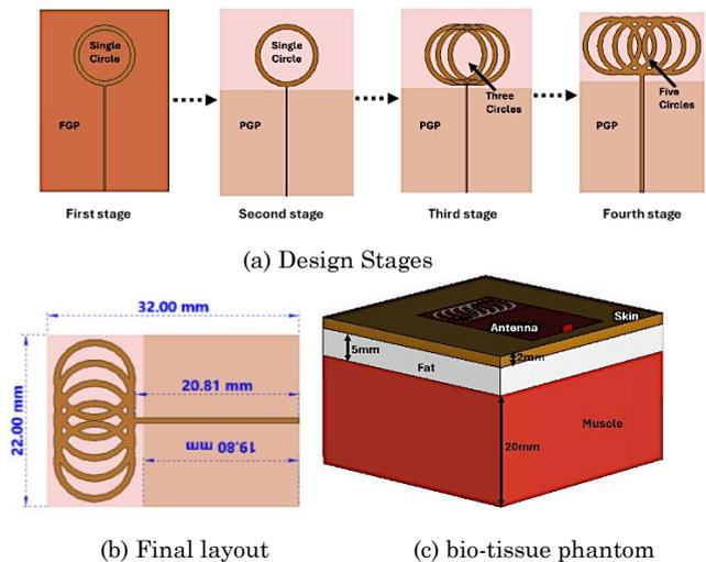
**Fig. 1** – The (a) stages of the proposed single antenna and the (b) final optimized structure of the antenna
