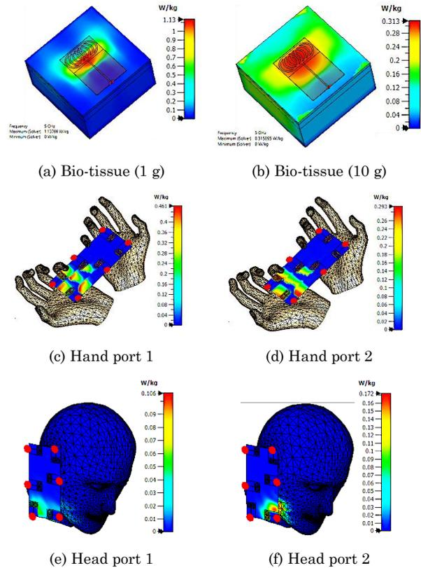
Fig. 7 – The SAR responses on different phantoms with SEA and MIMO
