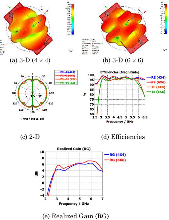
Fig. 5 – Far-field Radiation, efficiencies and the RG comparison between  $4 \times 4$  and  $6 \times 6$  MIMO
