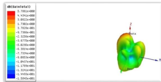
Fig. 5 – 3D gain for the final MIMO antenna design
