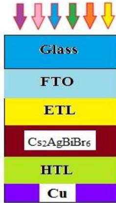
Fig. 1 – Device Structure used for Simulation
