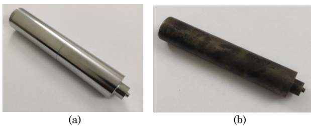
Fig. 5 – Tool (a) Before and (b) After heat treatment
