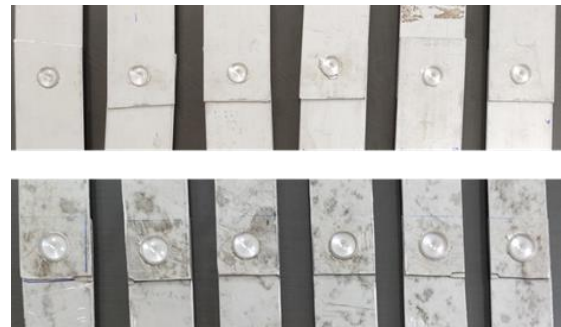
Fig. 4 – Manufactured FSSW specimen
