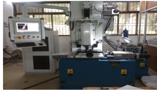
Fig. 3 – CNC linear friction stir welding machine
