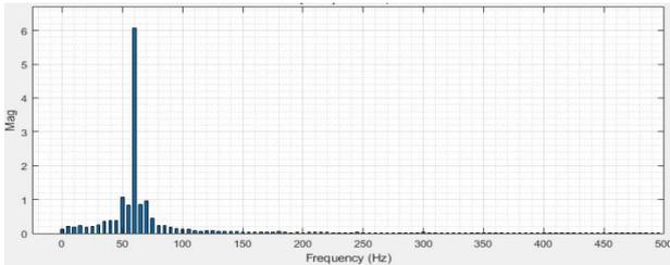
Fig. 4 – SPHBI's output current signal spectrum
