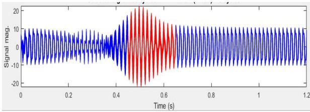
Fig. 2 – Collected SPHBI's output current signal
