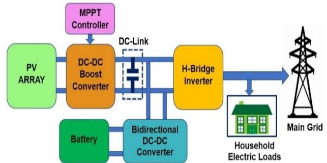
**Fig. 1** – Schematic diagram of the main grid-tied domestic MG PV system, an MPPT-driven DC/DC boost converter, a DC-link, a bidirectional DC/DC converter, a battery storage system, household electric loads and an SPHBI
