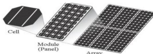
Fig. 1 – Solar PV cell, module and Array
