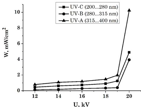
**Fig. 5** – Dependences of UV intensity – UV-C, UV-B, UV-A – discharge ranges on the voltage on the electrodes at  $f = 80$  Hz in argon between  $\text{Ag}_2\text{S}$  electrodes at a pressure of 101 kPa ( $d = 2$  mm)
