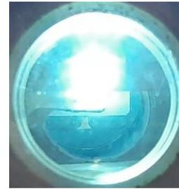
**Fig. 2** – View of an overvoltage nanosecond discharge between  $\text{Ag}_2\text{S}$  electrodes in atmospheric pressure argon at a discharge pulse repetition rate  $f = 1000$  Hz
