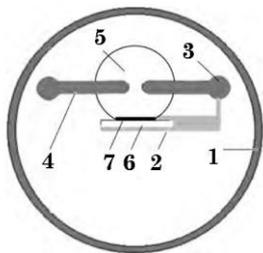
**Fig. 1** – Configuration of the discharge chamber: 1 – enclosure of the dielectric discharge chamber; 2 – substrate fixation mechanism for sputtering thin films; 3 – the apparatus for adjusting the interelectrode gap; 4 – metallic electrodes; 5 – region for film deposition; 6 – glass substrate; 7 – film structure
