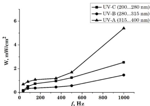
**Fig. 4** – Dependences of UV intensity – UV-C, UV-B, UV-A radiation – discharge ranges on the frequency of repetition of current pulses at a charging voltage of  $U = 13$  kV in argon between  $\text{Ag}_2\text{S}$  electrodes at a pressure of 101 kPa ( $d = 2$  mm)
