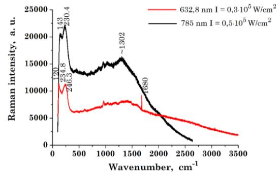
**Fig. 7** – Raman scattering spectrum of laser radiation at a wavelength of 785 nm by a thin film synthesized from electrode erosion products of an overvoltage nanosecond discharge between electrodes from the superionic conductor  $\text{Ag}_2\text{S}$  ( $p_{Ar} = 101$  kPa)
