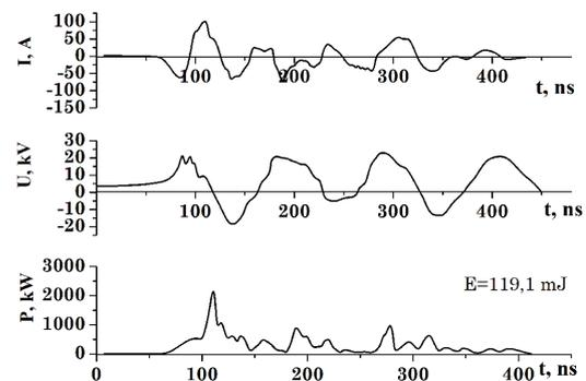
**Fig. 3** – Oscillograms of current and voltage pulses, pulsed power and energy contribution to an overvoltage nanosecond discharge per pulse ( $p_{\text{Ar}} = 101$  kPa,  $f = 1000$  Hz,  $d = 2$  mm)
