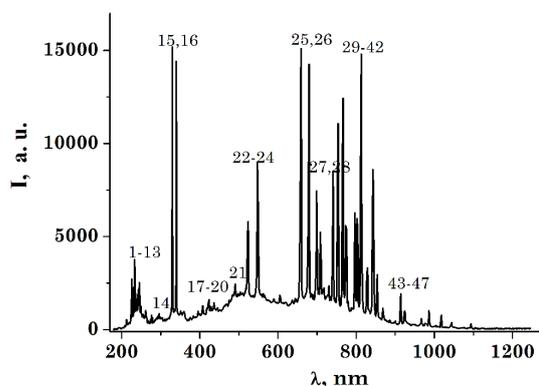
**Fig. 6** – UV-radiation spectrum of the discharge plasma between the electrodes from the  $\text{Ag}_2\text{S}$  compound at:  $p_{\text{Ar}} = 101$  kPa;  $f = 1000$  Hz,  $d = 2$  mm
