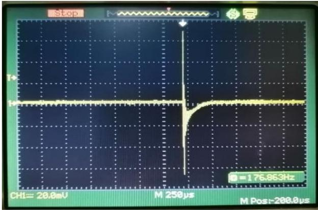
Fig. 9 – The lifetime measurements of charge carriers by open-circuit voltage decay photograph method for ZnO/P<sub>Si</sub>/p-Si
