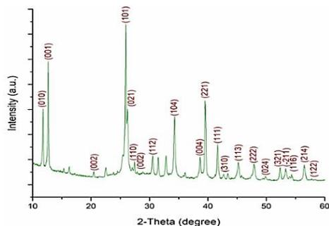
Fig. 1 – XRD of Fe<sub>2</sub>O<sub>3</sub>-FAPbI<sub>3</sub>-TiO<sub>2</sub> nanocomposite
