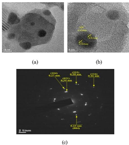
Fig. 2 – (a) TEM image of Fe<sub>2</sub>O<sub>3</sub>-FAPbI<sub>3</sub>-TiO<sub>2</sub> nanocomposite (b) HRTEM image of Fe<sub>2</sub>O<sub>3</sub>-FAPbI<sub>3</sub>-TiO<sub>2</sub> nanocomposite (c) SAED image of Fe<sub>2</sub>O<sub>3</sub>-FAPbI<sub>3</sub>-TiO<sub>2</sub> nanocomposite
