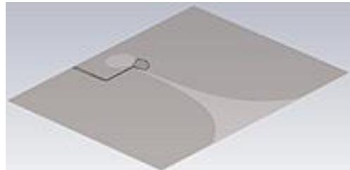
**Fig. 2** – Single Element Vivaldi Antenna
