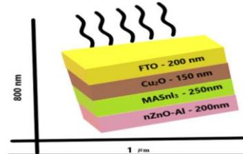
Fig. 1 – Solar PV structure FTO/Cu<sub>2</sub>O/MASnI<sub>3</sub>/nZnO-Al
