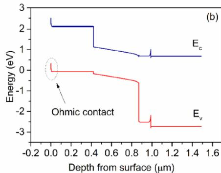
Fig. 6 – Band Diagram of PSC with ohmic contact.
