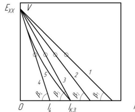
**Fig. 4** – The current-voltage characteristic of thermoelectric generator at  $Q = \text{const}$  and  $T_h = \text{const}$ : 1 – at  $T_h = \text{const}$  and  $T_c = \text{const}$ ; 2 and 4 – boundary; 3 – linearized; 5 – fine [11]
