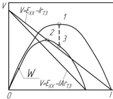
Fig. 5 – Dependence of the current-voltage characteristic in terms of power on the voltage and current of the thermoelectric generator [11]
