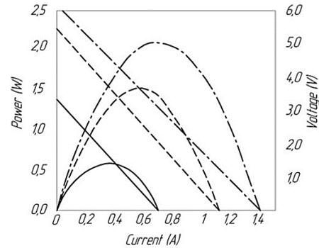
Fig. 6 – The current-voltage characteristic of thermoelectric generator at various surface temperature gradients ( $\Delta T$ ,  $^\circ\text{C}$ ): — 50; - - - 85; - · - 105
