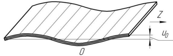
**Fig. 3** – A traveling electromagnetic flexural wave in an envelope plate:  $u_0$  is the displacement amplitude of the plate elements in a flexural wave, the *z* axis is the direction of wave propagation
