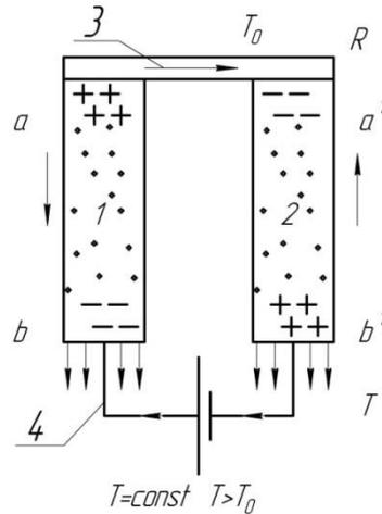
Fig. 1 – Battery of thermoelectric generator: 1, 2 – rods of conductors; 3 – connecting bridge; 4 – electrical circuit
