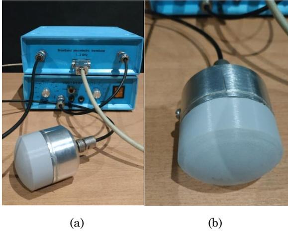
**Fig. 1** – Developed therapeutic device(a) and broadband plate piezo transducer(b)
