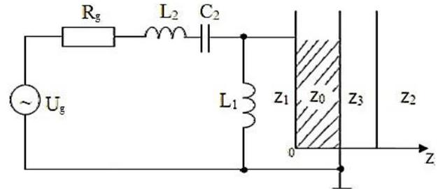
**Fig. 7** – Electroacoustic calculation scheme of a piezo element with a transition layer and electrical correction circuits
