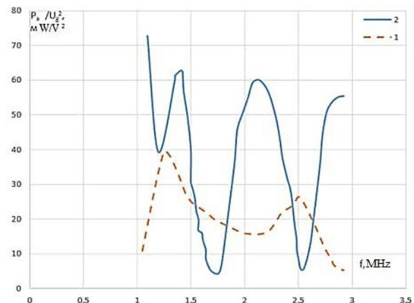
**Fig. 11** – Frequency response ratio  $P_a/U_g^2$  (curve 1) and the amount of current consumed at  $U_g = \text{const}$  (curve 2)
