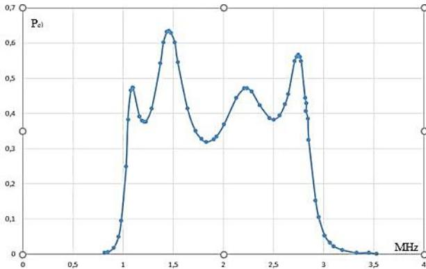
**Fig. 8** – Frequency response of the power transmission coefficient  $P_E$  piezo emitter for optimal matching layer thickness
