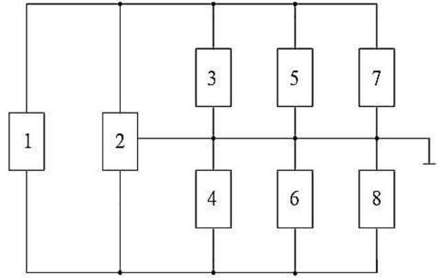
**Fig. 2** – Scheme of electrical structural measurement of the total electrical resistance module of the piezo transducer: 1 – generator; 2 – phase meter; 3 – frequency meter; 4 – oscilloscope; 5, 6 – voltmeter; 7 – ballast resistor; 8 – experimental sample
