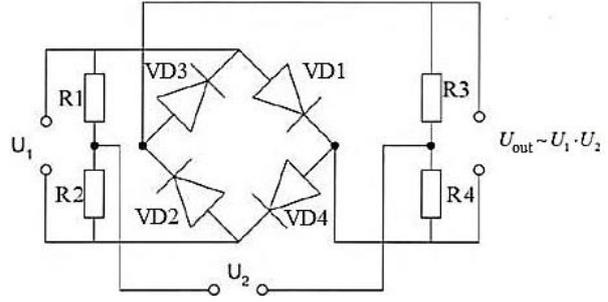
Fig. 4 – Ring balance circuit
