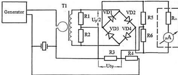
Fig. 5 – Practical diagram of a HF wattmeter with a piezo-emitter (PE)
