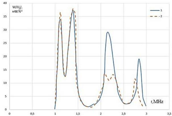
**Fig. 10** – Experimental frequency response of the ratio of the measured power to the square of the generator voltage, provided  $R_g = 0$  and close to the optimal emitter parameters
