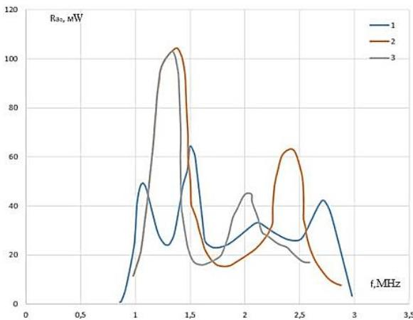
**Fig. 9** – Frequency dependence of the radiated power at a low value of the generator voltage
