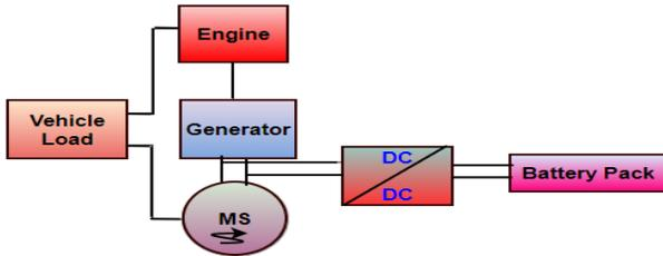
Fig. 1 – Structural Diagram of a hybrid electric vehicle (HEV)
