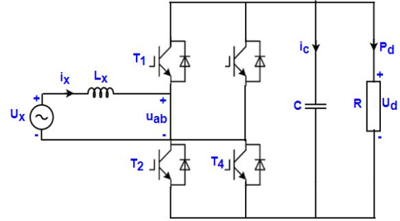
Fig. 2 – Circuit Diagram of a two-level with four quadrant converters
