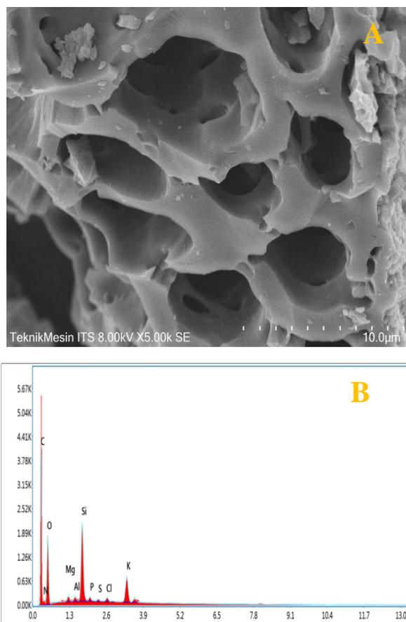
Fig. 1 – (A) SEM Image of corncob biochar (B) EDS spectrum of corncob biochar
