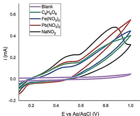
**Fig. 3** – CV Curve of CPE/CB electrode in 20 mg L<sup>-1</sup> of NO<sub>2</sub> solution and 20 mg L<sup>-1</sup> of various interferences in 0.1 M phosphate buffer, pH 7.0, scan rate 100 mV s<sup>-1</sup>
