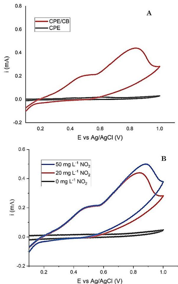
**Fig. 2** – (A) CV curves of CPE and CPE/CB modified electrode in a 0.1 M phosphate buffer (PH = 7) solution containing 20 mg L<sup>-1</sup> NO<sub>2</sub> at a scan rate of 100 mV s<sup>-1</sup>, (B) CV Curve response of CPE/CB electrode in 0, 20 and 50 mg L<sup>-1</sup> NO<sub>2</sub>
