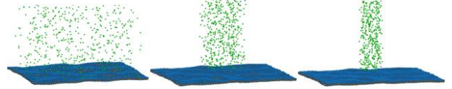
Fig. 2 – Initial atomistic configuration of the system, consisting of Ti 2 C MXene and Ag atoms with three different sizes of surface growth areas: 20 × 17, 6.0 × 6.0 and 3.0 × 3.0 nm 2 from left to right
