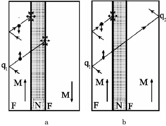
**Fig. 1** – Schematic representation of the spin-polarized transport of charge carriers in a sandwich with *ap* – configuration (a) and *p* – configuration (b) in the assumption that the main (responsible for the effect) electrons are charge carriers whose spin direction coincides with the direction of the spontaneous magnetization vector in magnetic metal layers (majority spin-polarized electrons)
