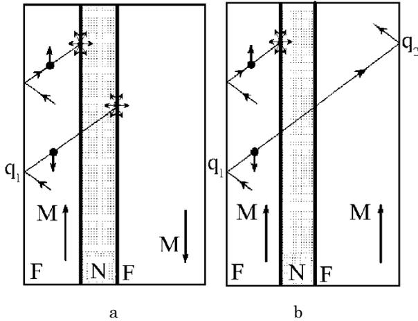
**Fig. 2** – Schematic representation of the spin-polarized transport of charge carriers in a sandwich with *ap* – configuration (a) and *p* – configuration (b) in the assumption that the main (responsible for the effect) electrons are charge carriers whose spin direction is opposite to the direction of the spontaneous magnetization vector in magnetic metal layers (majority spin-polarized electrons)
