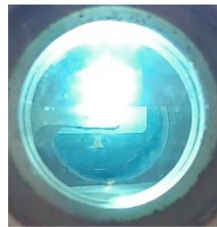
**Fig. 2** – View of an overvoltage nanosecond discharge between two polycrystalline electrodes made of a superionic conductor at a distance between the electrodes  $d = 2$  mm and a current pulse repetition rate  $f = 1000$  Hz
