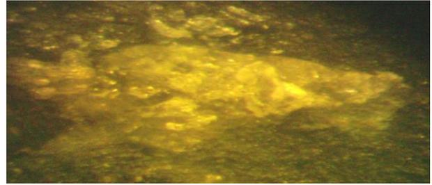
**Fig. 2** – SiO<sub>2</sub> surface after nanosecond laser irradiation by the ruby laser with the intensity  $I \approx 400$  Mw/cm<sup>2</sup> with the dose  $D = 5 \times I$  and the ruby laser pulse duration  $\tau \approx 20$  ns with the wavelength  $\lambda = 694$  nm ( $\times 98$ )
