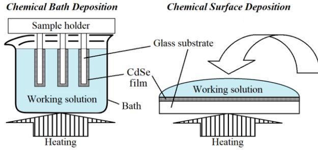
**Fig. 1** – The scheme of obtaining CdSe films by CSD and CBD methods
