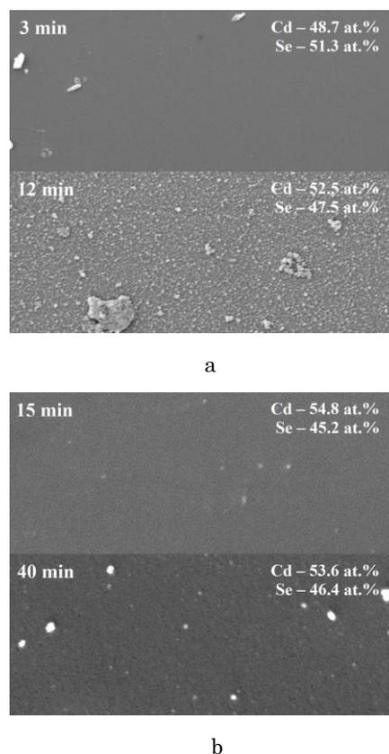
**Fig. 4** – Surface morphology ( $\times 5000$  magnification) and atomic composition of CdSe films obtained by CSD (a) and CBD (b) methods at various process durations
