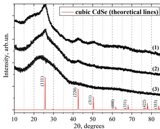
**Fig. 3** – Experimental XRD patterns of CdSe films on glass substrates obtained by CSD (1) and CBD (2) methods and XRD pattern of a glass substrate (3) without CdSe film for comparison
