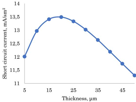
Fig. 4 – Dependence of the short circuit current of *p-i-n* amorphous silicon solar cell on the base thickness
