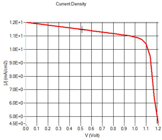
**Fig. 1** –  $I$ - $V$  characteristic of a  $p$ - $i$ - $n$  amorphous silicon solar cell:  $d_n = 200$  nm,  $d_p = 200$  nm,  $d_i = 5$   $\mu$ m,  $N_A = 1e16$  cm $^{-3}$ , and  $N_D = 1e17$  cm $^{-3}$
