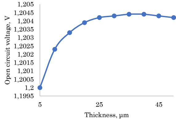
**Fig. 3** – Dependence of the open-circuit voltage of a  $p$ - $i$ - $n$  amorphous silicon solar cell on the base thickness
