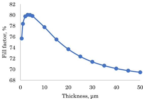
Fig. 5 – Dependence of the fill factor of *p-i-n* amorphous silicon solar cell on the base thickness
