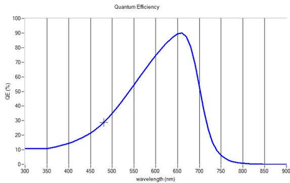
**Fig. 2** – Quantum efficiency of a  $p$ - $i$ - $n$  amorphous silicon-based solar cell. Here,  $d_n = 200$  nm,  $d_p = 200$  nm,  $d_i = 5$   $\mu$ m,  $N_A = 1e16$  cm $^{-3}$  and  $N_D = 1e17$  cm $^{-3}$
