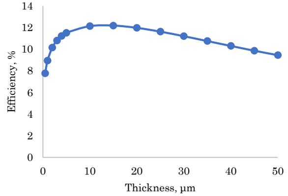
Fig. 6 – Dependence of the efficiency of *p-i-n* amorphous silicon solar cell on the base thickness
