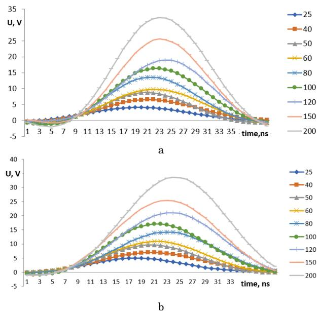
**Fig. 3** – Typical amplitude-time characteristics of switching for samples of series 1 (a) and 2 (b) when changing the maximum amplitude of a pulse from 25 to 200 V
