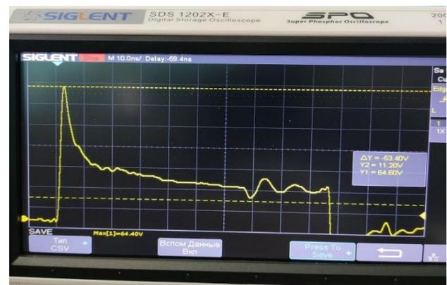
Fig. 2 – Volt-second characteristic of the switching process in a cadmium telluride film
