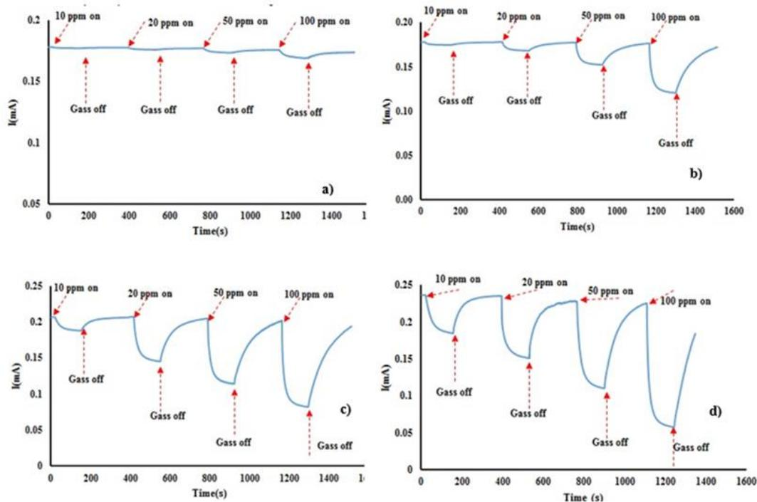
Fig. 4 – Variation of current with time for CNT with catalyst (Fe) for CO<sub>2</sub> with different concentrations and temperatures
