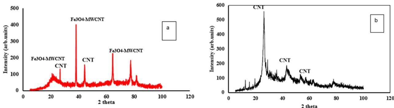
Fig. 2 – XRD of CNT a) with catalyst (Fe) and b) without catalyst (purity)
