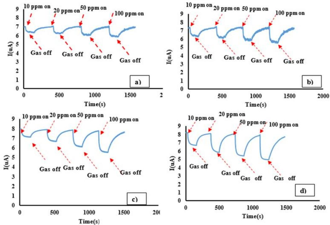
Fig. 3 – Variation of current with time for CNT without catalyst (purity) for CO<sub>2</sub> with different concentrations and temperatures
