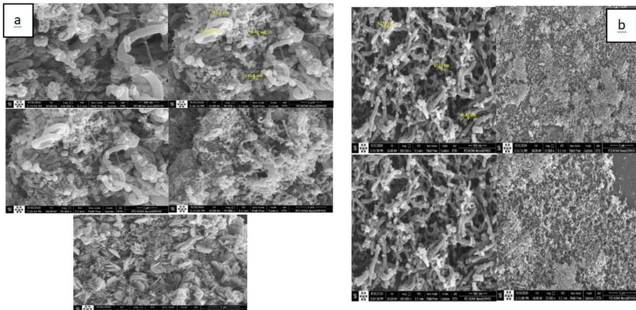
Fig. 1 – FESEM images of CNT a) with catalyst (Fe) and b) without catalyst (purity)
