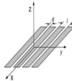
Fig. 1 – Diffraction grating
