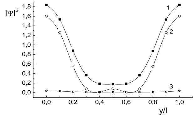
Fig. 2 – Diffraction patterns of distribution  $|\Psi|^2$  at different values of the fill factor  $d/l$ : 1 – 0.9; 2 – 0.5; 3 – 0.1; at  $l/\lambda = 1.9$
