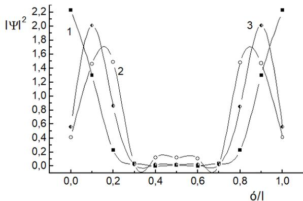
**Fig. 3** – Diffraction patterns of distribution  $|\Psi|^2$  at different values of  $l/\lambda$ : 1 – 2.1; 2 – 3.1; 3 – 4.1; at  $d/l = 0.5$
