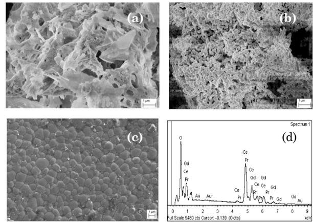
**Fig. 3** – SEM images of the PGDC sample at (a) 600 °C, (b) 1000 °C, (c) 1250 °C, and (d) EDS
