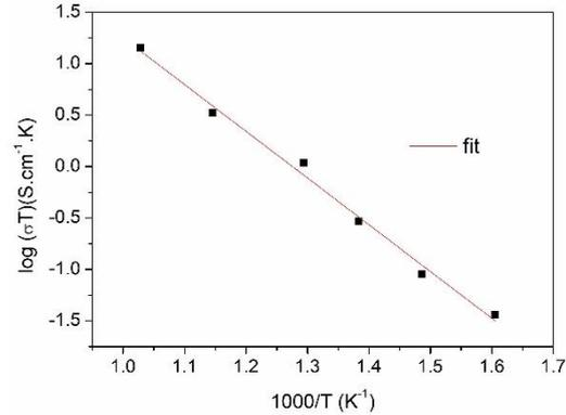
**Fig. 6** – Electrical conductivity versus  $1000/T$  of the PGDC sample
