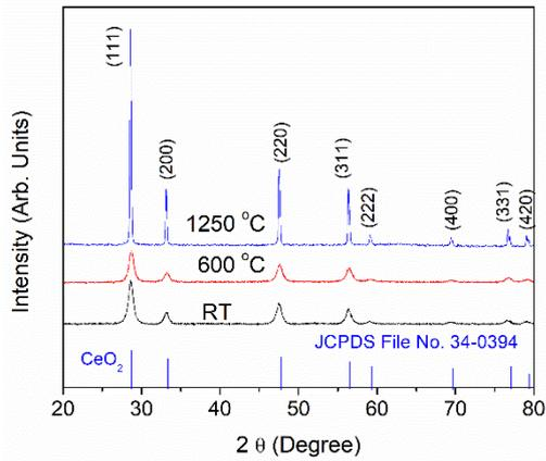
**Fig. 1** – XRD patterns of the PGDC powder samples at different temperatures
