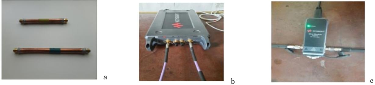
Fig. 1 – a) Segment of a coaxial line, b) vector network analyzer, c) automatic calibration tool
