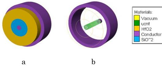
**Fig. 1** – 3D structure of GAA CNTFET (a) and a separate display of its channel and gate (b)
