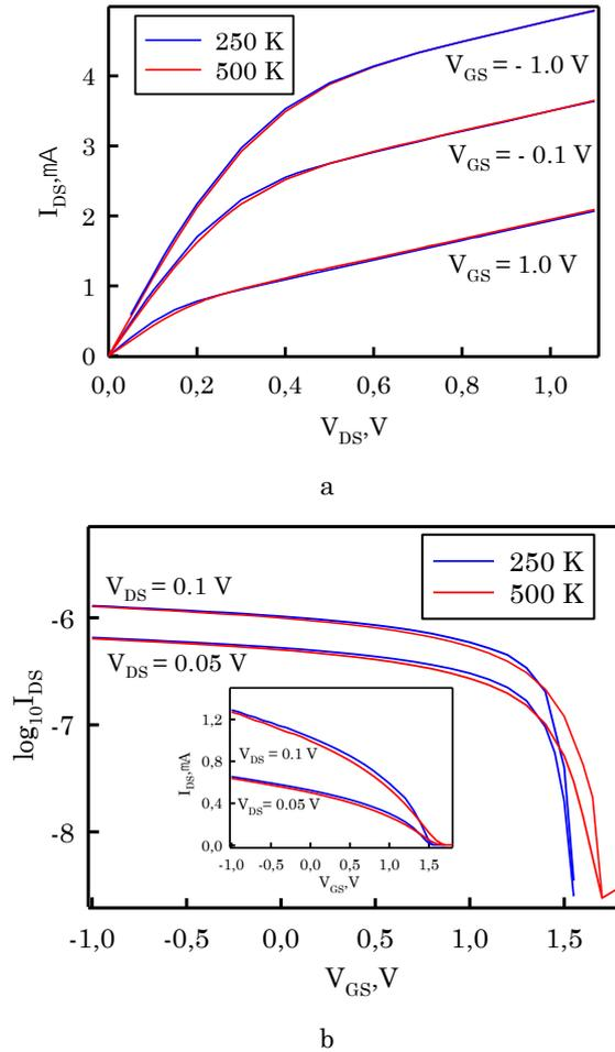
**Fig. 3** –  $I_{DS}$  (a) and  $I_{DS}$ - $V_{DS}$  (b) curves of  $n$ -type GAA CNTFET as a function of temperature variation
