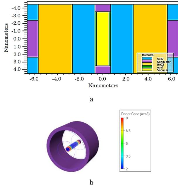
**Fig. 2** – Structure of GAA CNTFET: a – 2D structure of GAA CNTFET with channel and gate lengths of 7 nm and 5 nm, respectively; b – 3D structure of GAA CNTFET with impurity concentration distribution in the channel
