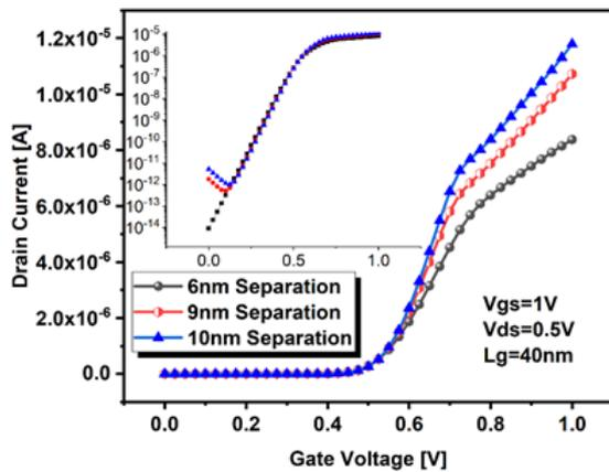
**Fig. 4** – Transfer characteristic of the proposed structure for different channel separation distances
