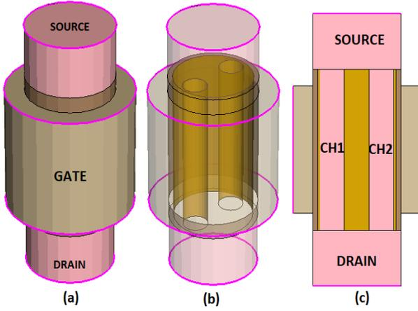
**Fig. 1** – (a) 3D structure, (b) internal structure, (c) cross-sectional view of a high- $k$  dielectric based on multi-channel GAA MOSFET structure
