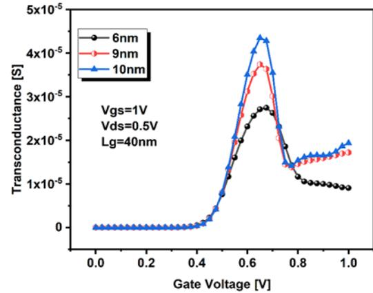
**Fig. 5** – Transconductance of the proposed structure for different channel separation distances
