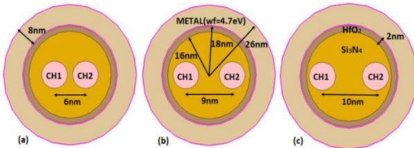
**Fig. 2** – (a) 3D structure, (b) internal structure, (c) cross-sectional view of a high- $k$  dielectric based on multi-channel GAA MOSFET structure
