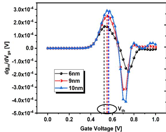
**Fig. 6** – Threshold voltage extraction of the proposed structure for different channel separation distances
