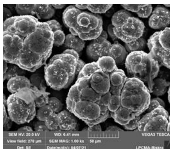
Fig. 2 – Surface morphology of Ni-P-TiO 2 composite coatings electrodeposited at different current densities (in \text{A dm}^{-2} ): (a) 2, (b) 3, (c) 4, (d) 5, and (e) 7
