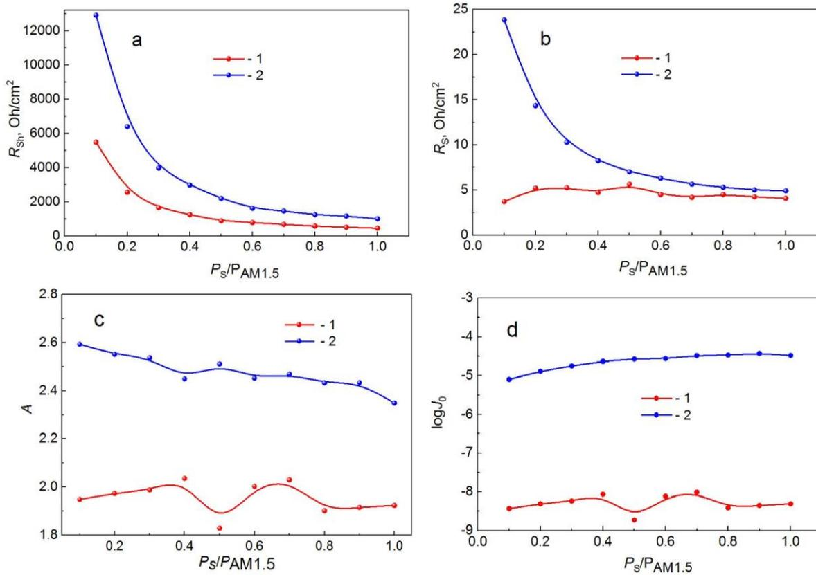
**Fig. 3** – Dependences of the diode parameters on the illumination level of the studied samples: 1 – SC with a nanoscale Cu layer in glass/FTO/CdS/CdTe/Cu/Au back contact, 2 – SC without a nanoscale Cu layer in glass/FTO/CdS/CdTe/Au back contact
