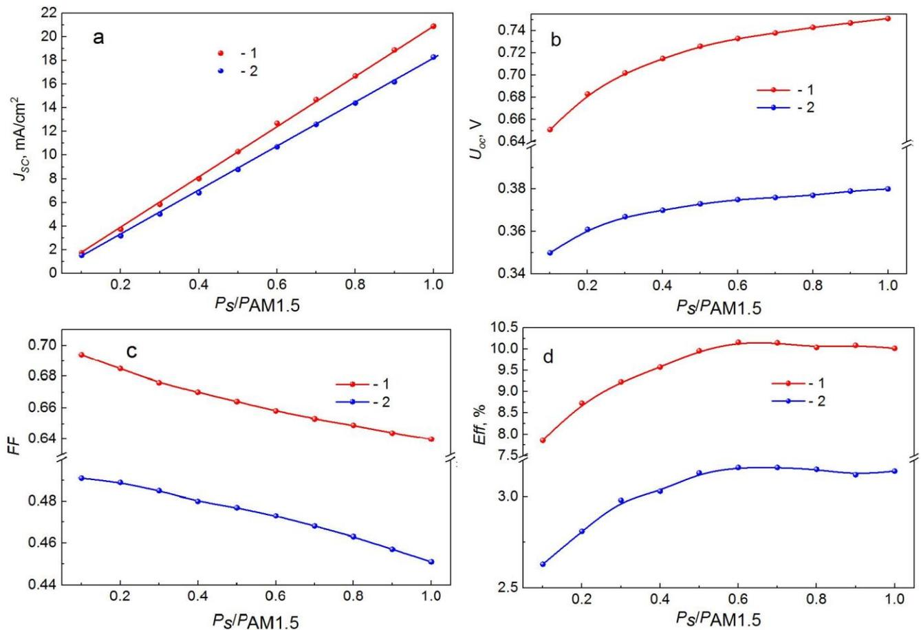
**Fig. 2** – Dependences of the output characteristics on different illumination levels of the investigated samples for: 1 – SC with nanoscale Cu layer in glass/FTO/CdS/CdTe/Cu/Au back contact; 2 – SC without nanoscale Cu layer in glass/FTO/CdS/CdTe/Au back contact
