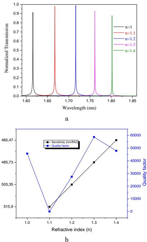
**Fig. 2** – Normalized transmission spectrum of the PhC sensor for different refractive indices ranging from  $n = 1$  to  $n = 1.4$  with an increment of  $\Delta n = 0.1$  (a), the calculated sensitivity and Q-factor of the proposed biosensor (b)
