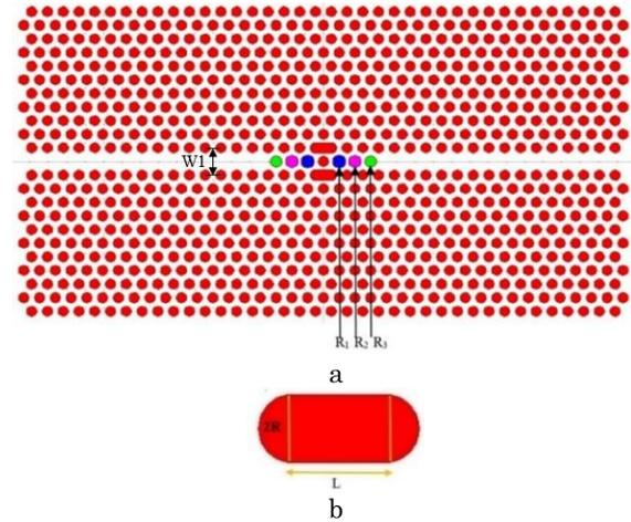
**Fig. 1** – Schematic of the capsule-shaped 2D-PhC sensor (a), geometrical parameters of the capsule-shaped cavity, namely  $L$  and  $R$  (b)
