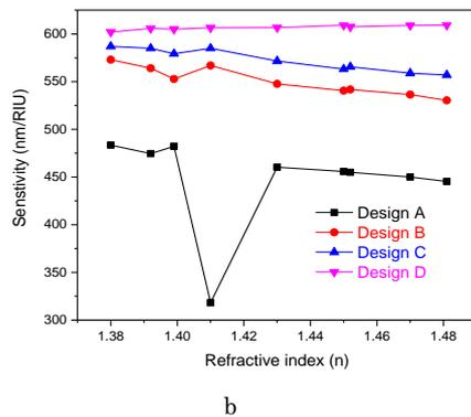
**Fig. 6** – Resonant wavelength variations depending on changes in the refractive index for four designs (a), the calculated sensitivity of the proposed four designs (b)
