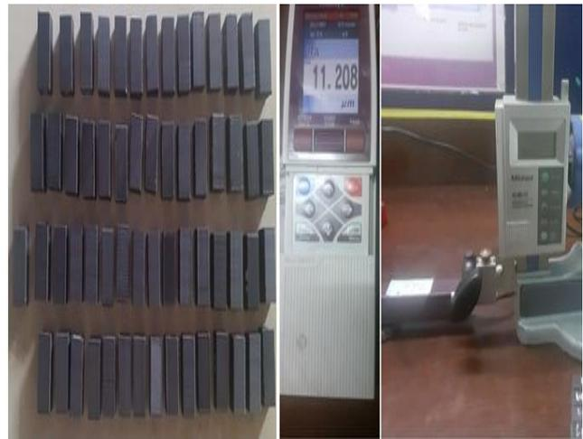
Fig. 1 – FDM fabricated test pieces and surface roughness measuring Mitutoyo Talysurf instrument
