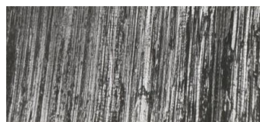
Fig. 5 – Appearance of the surface of a HRC steel ball counter after single-phase friction test: sliding velocity V = 14 m/s (a); V = 12 m/s (b); V = 8 m/s (c)
