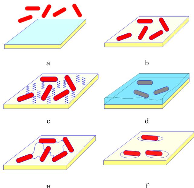
**Fig. 3** – Methods used for bioreceptor immobilization in biosensors: before immobilization (a), adsorption (b), covalent binding (c), matrix entrapment (d), cross-linking (e), encapsulation (f)
