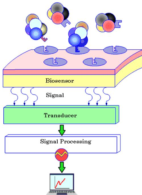
**Fig. 1** – Diagram of the structure and operating principle of biosensors
