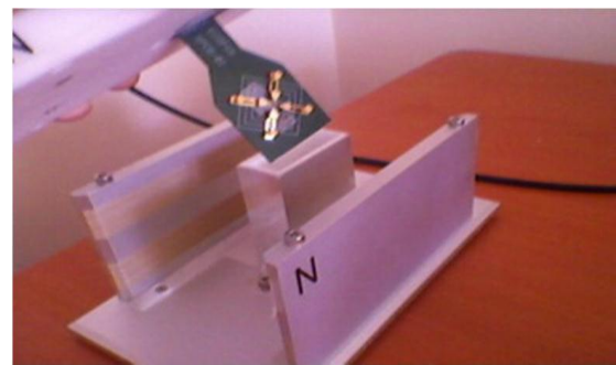
Fig. 7 – Hall measurement apparatus of undoped ZnO and Fe-doped ZnO. The films are kept by four Au probes as signed by the arrow
