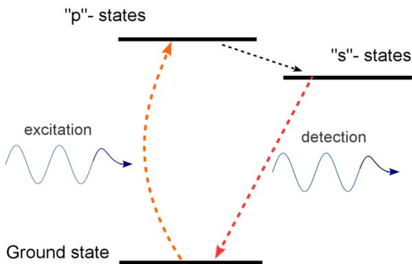
**Fig. 1** – Measurement of the photoluminescence from the  $s$ -level provides a measure of the final  $p$ -level occupation
