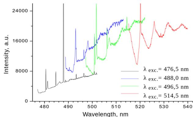
Fig. 3 – Raman spectroscopy spectra and photoluminescence of CdSe nanoparticles at different excitation wavelengths
