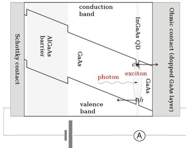
**Fig. 2** – Principle of exciton population photocurrent detection. An electric field is applied between the contacts of the photodiode and due to this, the carriers tunnel from the dot. This is reflected in the change of the current (for instance, if the excitation laser repetition rate is 76 MHz, the  $\Delta I$  will be 12.18 pA)
